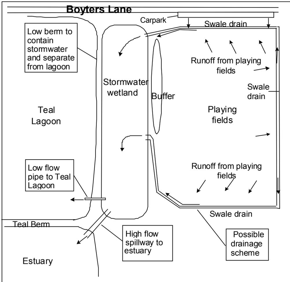
**Figure 4: Potential layout of a stormwater wetland showing likely flow patterns**
