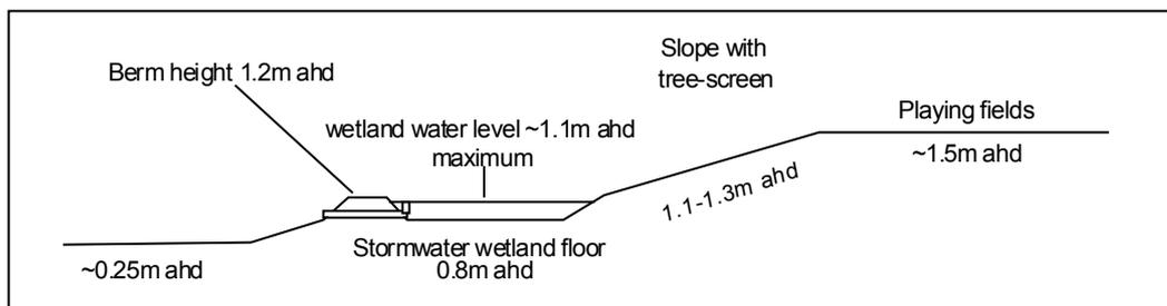
**Figure 5: Simple elevation layout of proposed stormwater wetland**
