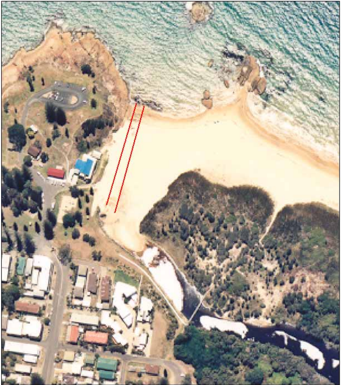
Figure C-4 Approximate position of pilot channel for inducing artificial breakout
