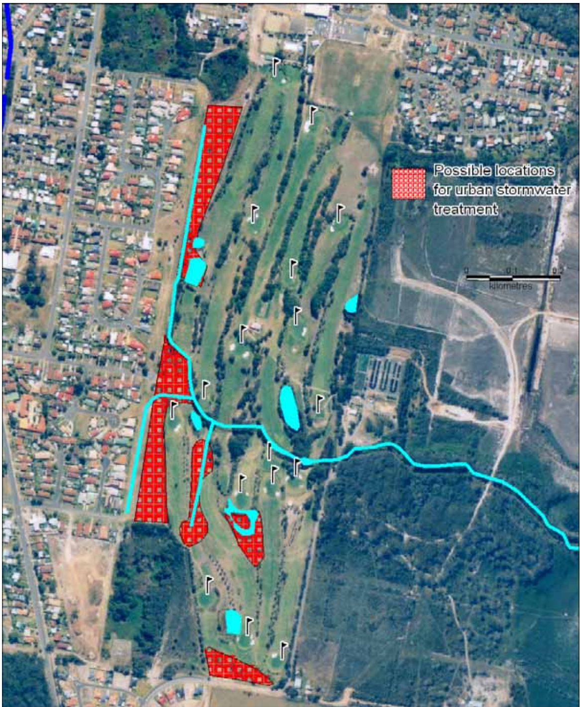
Figure 6-6 Possible location and configuration of wetlands and stormwater treatment devices within the South West Rocks Country Club
