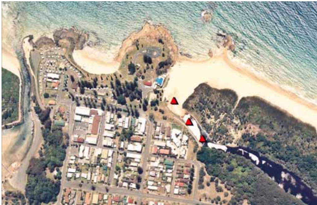
Figure C-2 Suggested locations for minimum water quality monitoring to assess entrance breakout requirements
