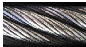
Right hand Lang's lay (RHLL) wire rope strands are twisted to the right like a screw conventional thread
