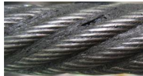
Left hand ordinary lay (LHOL) wire rope strands are twisted to the left
