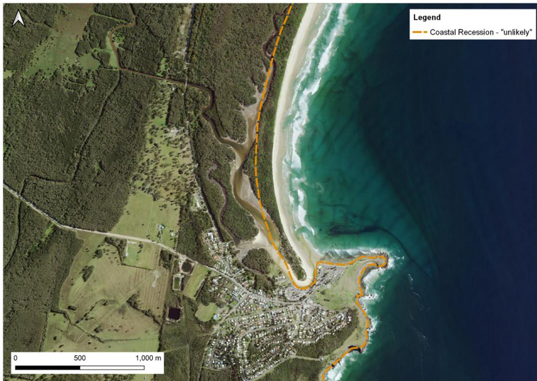
Figure 3-4: Combined coastal recession and beach erosion under a 2100 scenario at Crescent Head
