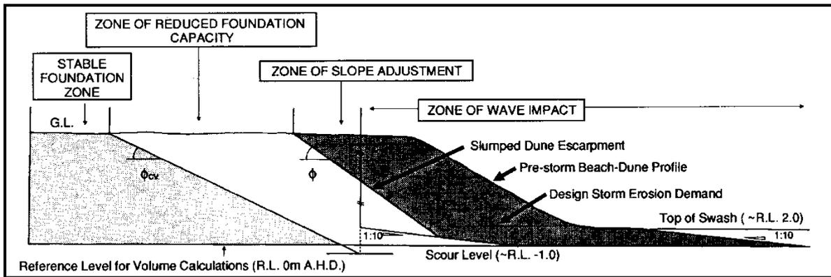
Figure 3-24 Design Profile and zones of instability for Storm Erosion (From Nielsen *et al.*, (1992))
