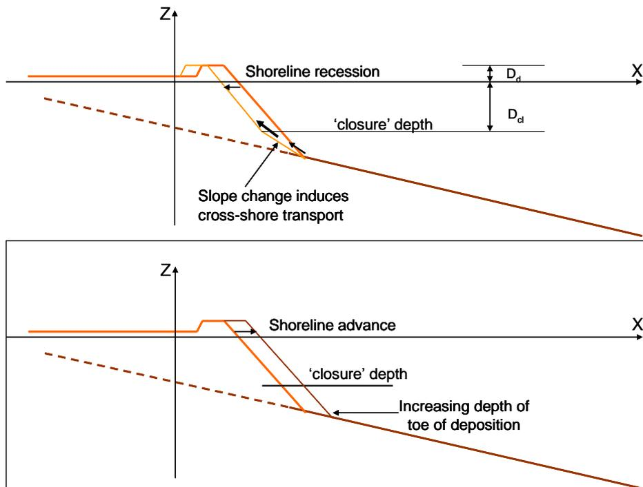
Figure 3-11 Cross shore schematisation of upper profile change for receding (top) and advancing (bottom) shoreline (Patterson, 2010)
