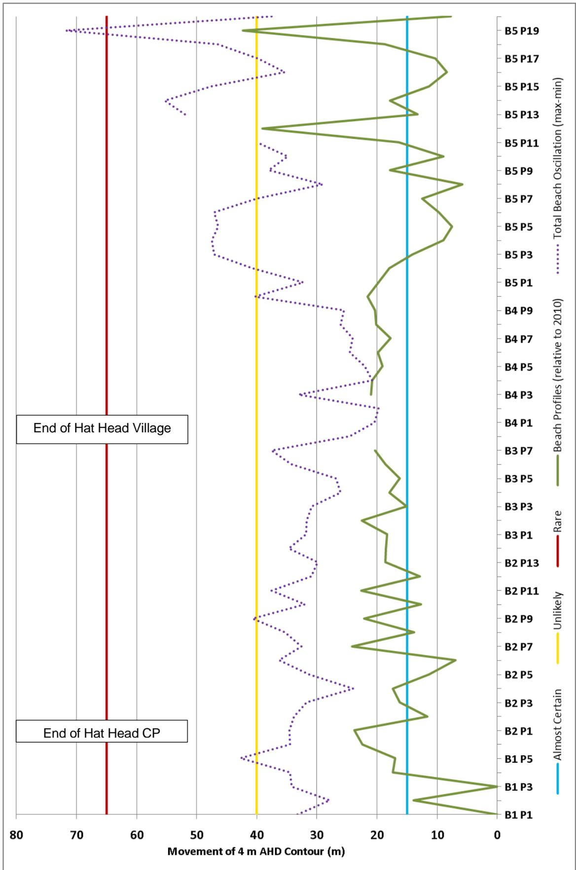
Figure 3-5 Beach Erosion Calculation, Hat Head Beach (with notation of photogrammetric block B and profile P)
