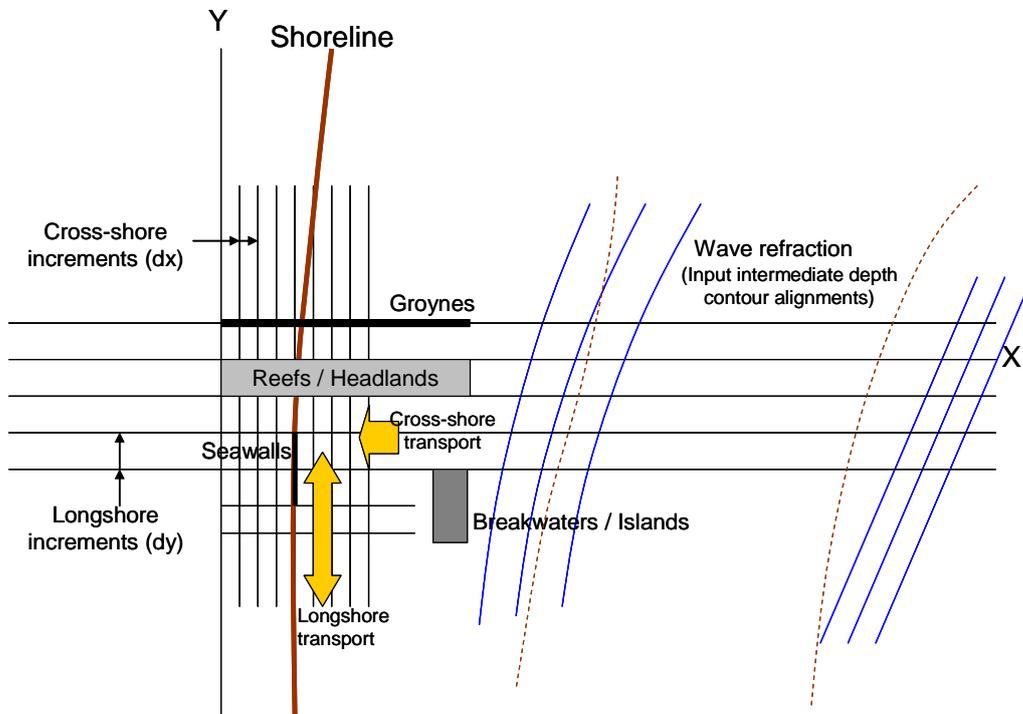
Figure 3-10 Plan view schematisation of SEM domain (Patterson, 2010)
