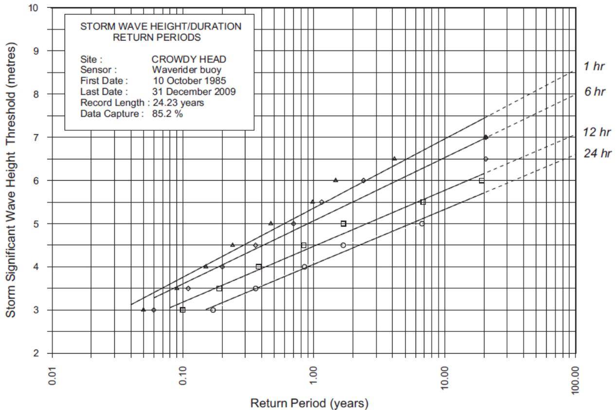
**Figure 2-6 Storm Wave Height / Duration Curves for the Crowdy Head Waverider Data**
