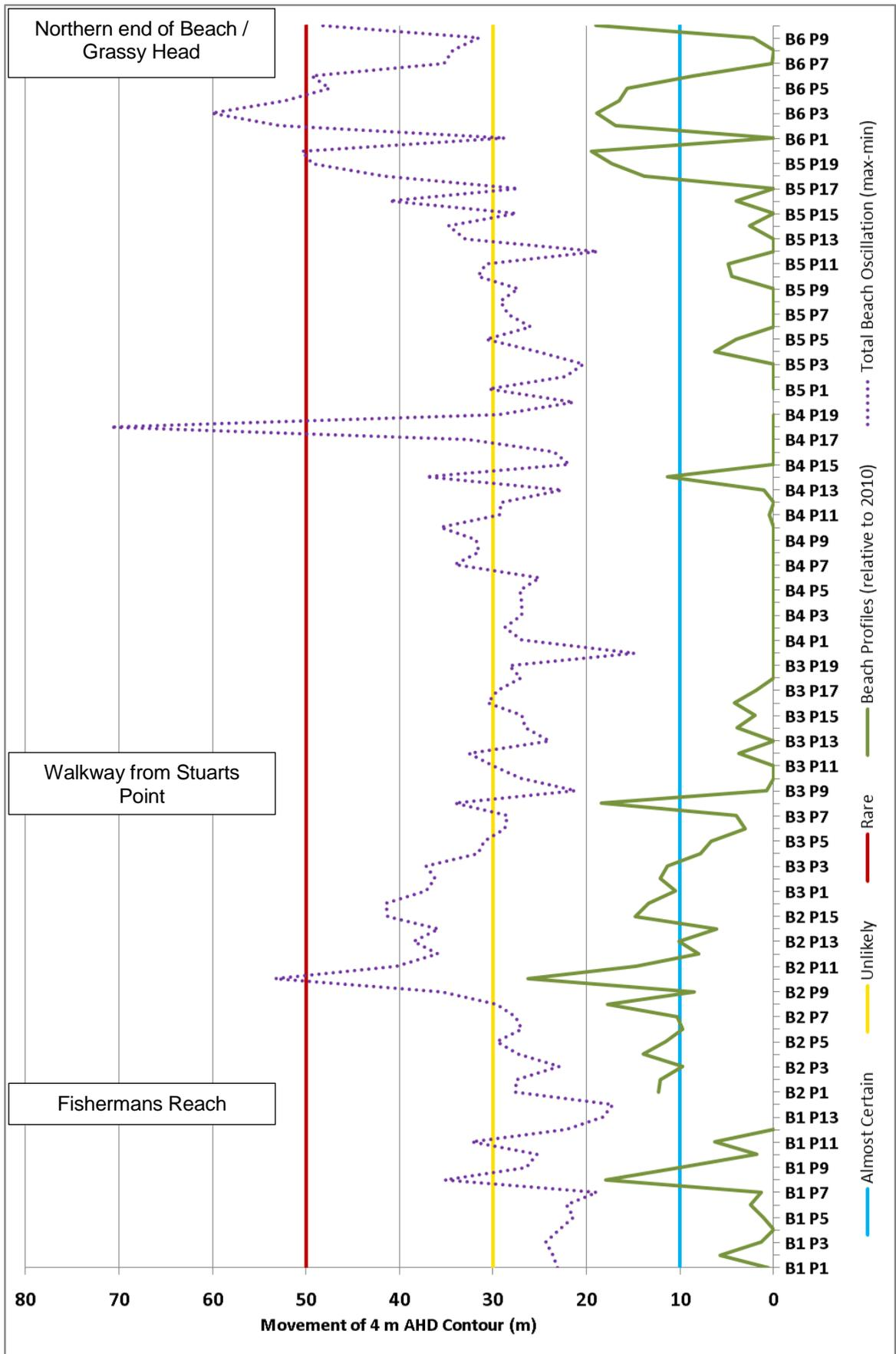
Figure 3-6 Beach Erosion Calculation, Stuarts Point Beach (with notation of photogrammetric block B and profile P)
