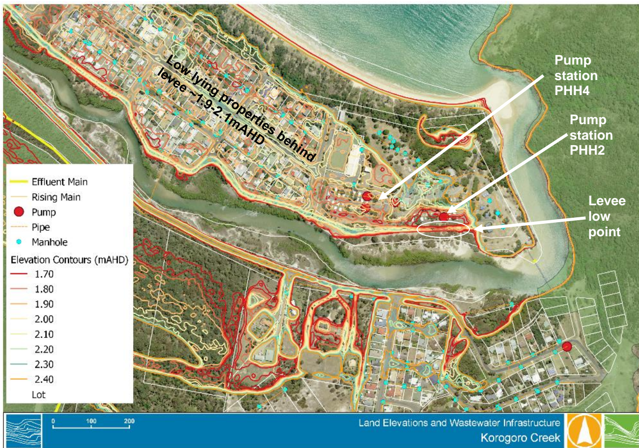
Figure 5-7 Local topographic contours and wastewater assets
