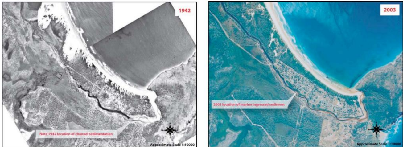
Figure 5-2 Comparative aerial photographs showing the flood tide delta in 1942 (left) and 2003 (right), showing marine sands pushed through the entrance (source: GECO Environmental, 2009b)
